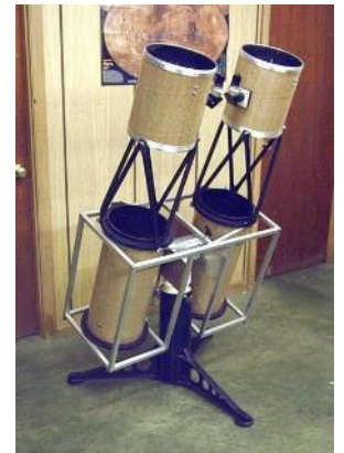
8" binocular telescope built by John Mahony, Jim Sattler, and Jim Mettler
