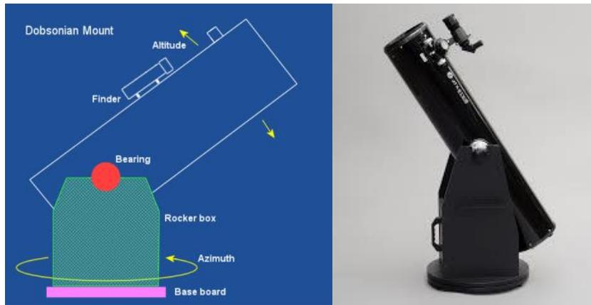
The design of the Dobsonian mount is, again, simple and, again, helps keep down the overall cost of the telescope. It is an “alt-az”, i.e., altitude-azimuth design. Altitude is how high up or down the telescope is pointed, azimuth is the horizontal angle of a compass bearing, i.e. it’s swinging the telescope to the left or right.
